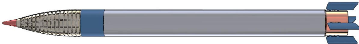
Fig. 1: 122 mm air-to-surface unguided rocket with prefragmented HE warhead
